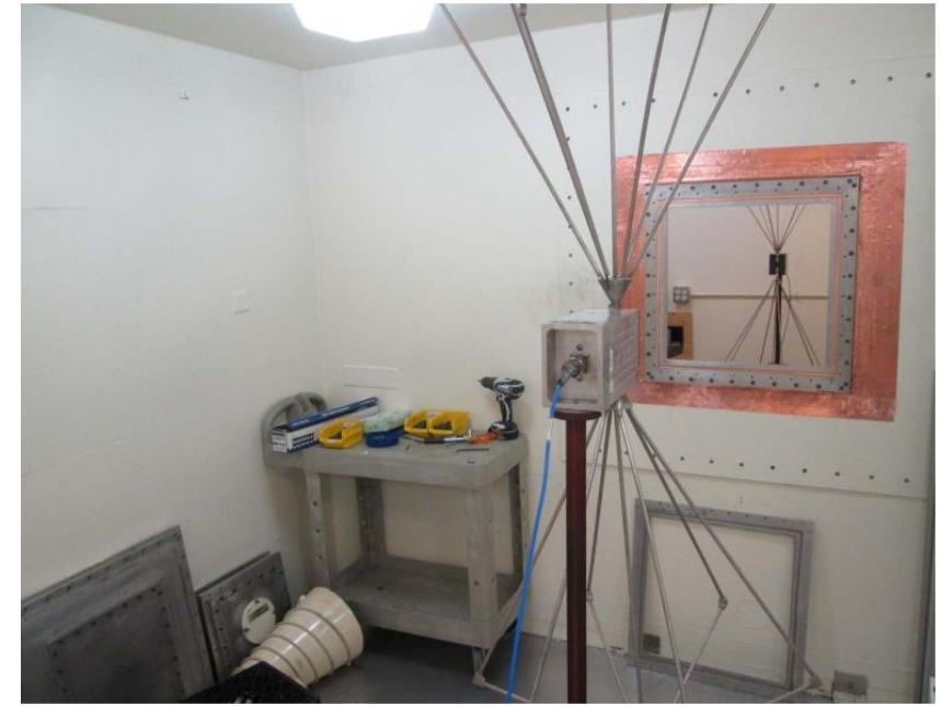
IEEE 299 dual chamber setup
