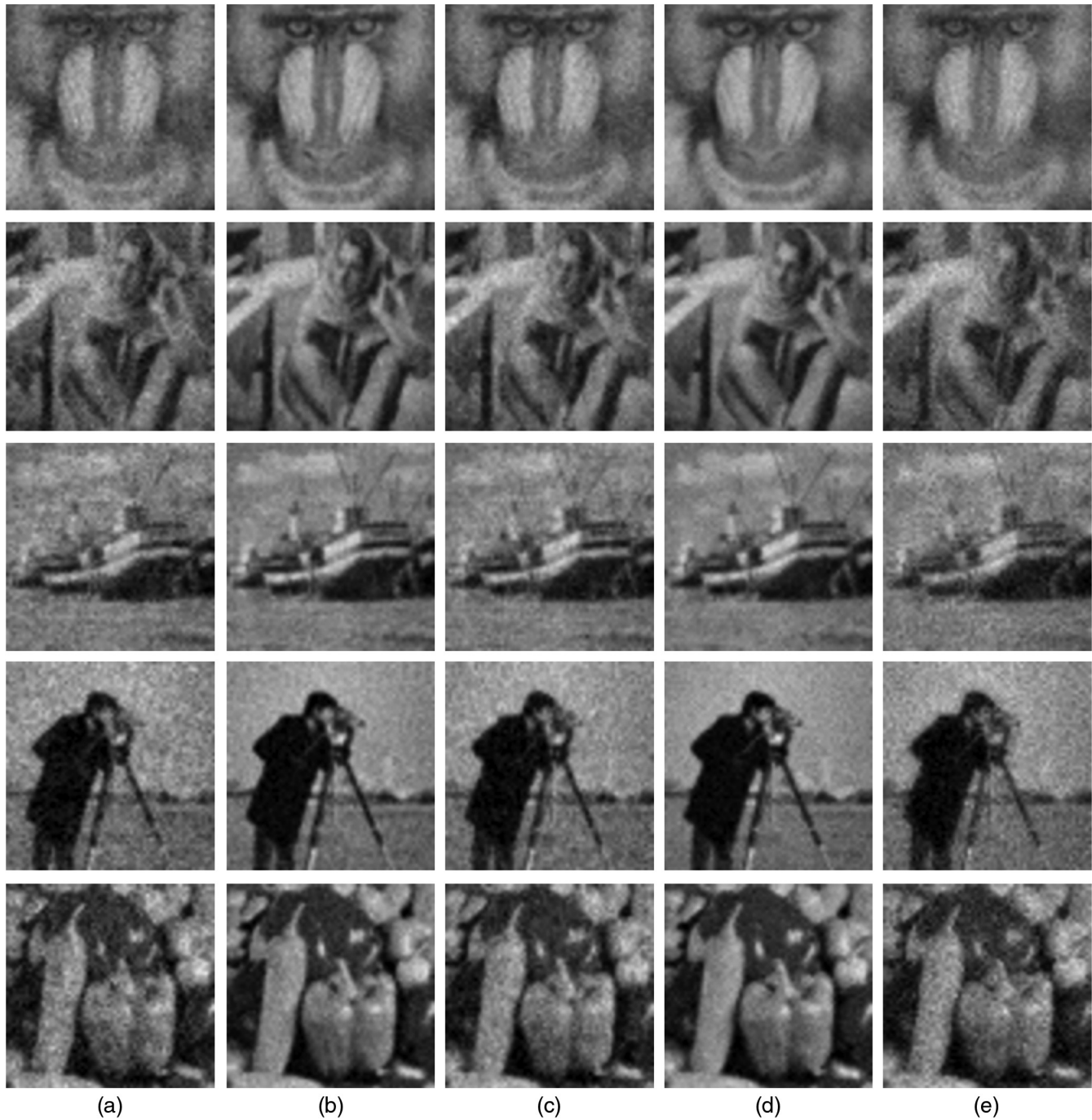
Fig. 6 Reconstructed images from 50% compressive measurements using (a) l_1 -norm minimization, (b) RefCS using low-resolution (25%) references, (c) RefCS using low-resolution (6.25%) references, (d) RefCSLS using low-resolution (25%) references, and (e) RefCSLS using low-resolution (6.25%) references.
