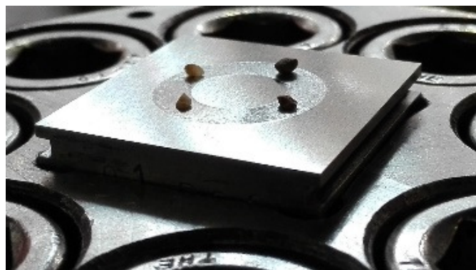
Figure 13- Sand Placement on HPT Sample.
