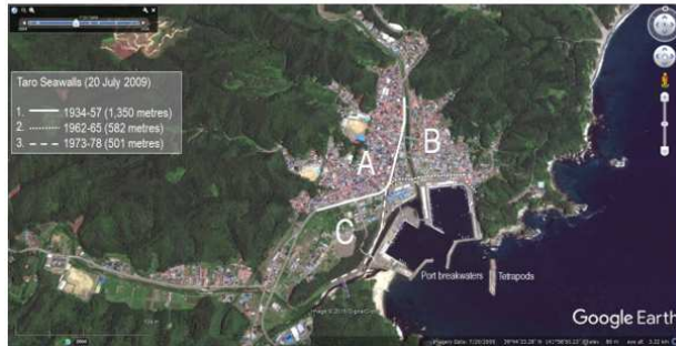
Figure 3. Google Earth Pro historical image of Tarō on 20 July 2009, with pre-2011 seawalls superimposed. Image compiled by the authors.
