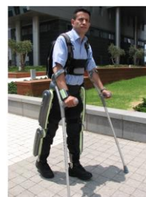
Fig. 1. The ReWalk Personal with an immobilized person inside [2].
