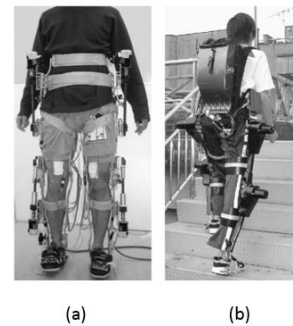
Fig. 6. HAL robotic exoskeleton, (a) the first prototype HAL-1, and (b) the second product HAL-3 [19].
