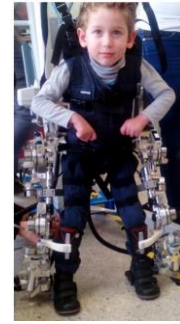
Fig. 8. ATLAS 2020, worn by a disable user [28].
