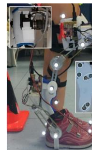
Fig. 9. The details of the WAKE-up system with joint modules and shoe pad [32].
