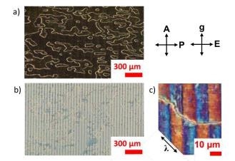
**Figure 4**. The texture of the SmC\* in a) the OFF, and b) the ON state; c) the two opposite twists of the SmC\* **c**-director in the presence of an electric field across an IDE and over a defect line.
