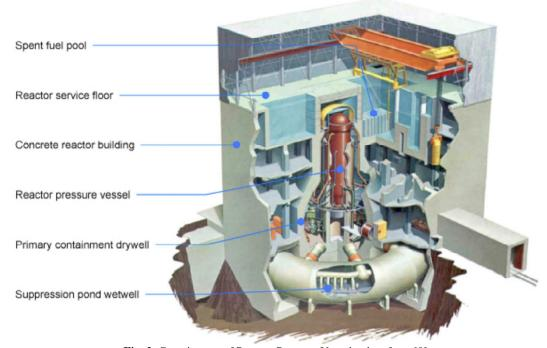
Fig. 2. Containment of Reactor Pressure Vessel, taken from [9].
