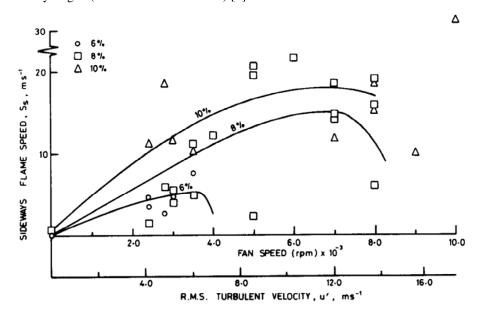
Fig. 1. Quenching effect of the rms turbulent velocity on hydrogen-air flame speed, taken from [4].
