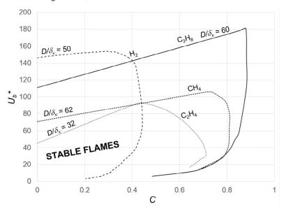
Fig. 4. Blow-off limits of stable CH<sub>4</sub>, C<sub>2</sub>H<sub>4</sub> and C<sub>3</sub>H<sub>8</sub>, lifted flames with air cross flows, in terms of  $U_b^*$  versus C, for different values of  $D/\delta_c$ . The dashed curve for H<sub>2</sub> is synthesised from the data of the other fuels.
