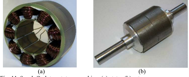
Fig. 11. 8-pole/9-slot prototype machine. (a) stator (b) rotor.
