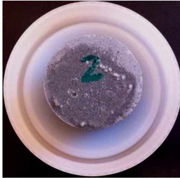
Fig. 5. Large and transparent efflorescence products appear on the drying top surface of GPC-NH 2 after 3 hours in contact with water at bottom.
