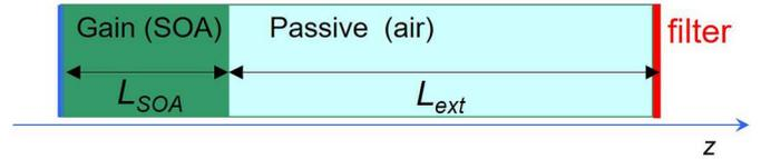
Fig. 1. Schematic of the simulated laser geometry.
