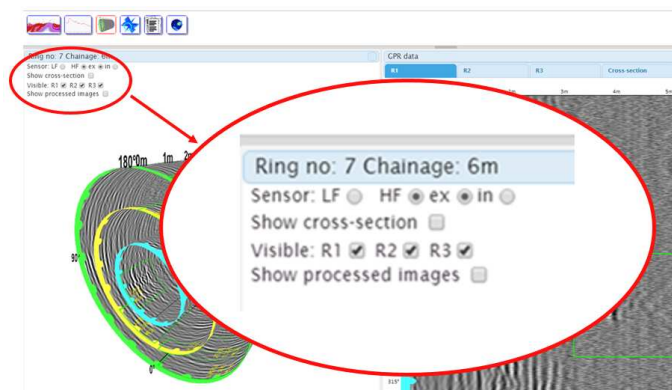
Figure 10: GPR visualisation options. Users can switch between different GPR sensors and different data capturing radii.
