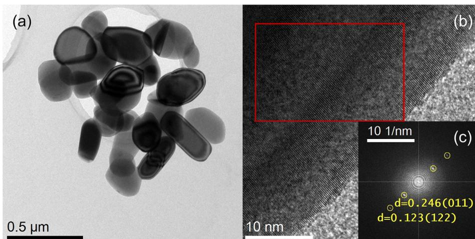
**Fig. 1.** (a) TEM image of  $\text{TiO}_2$  particles after milling for 1 min. (b) High magnification image of a  $\text{TiO}_2$  nanoparticle after 1 min of milling to show the lattice fringes. (c) Fast Fourier transform (FFT) generated from the red square shown in (b), with measured d-spacings in nm and corresponding hkl planes shown referenced to the rutile crystal structure [62].
