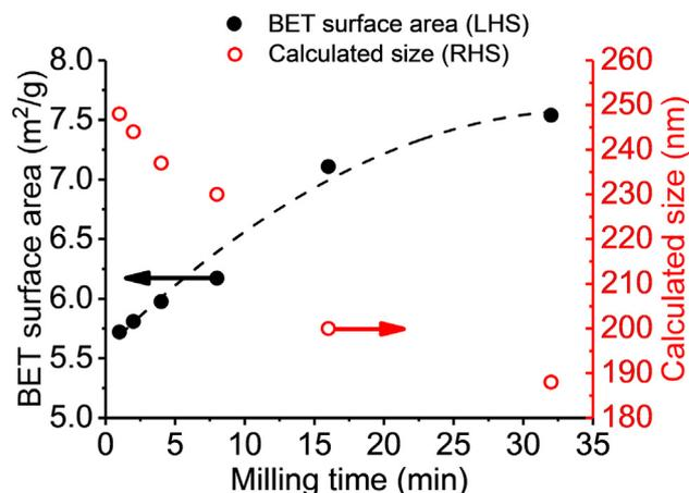
**Fig. 9.** Brunauer–Emmett–Teller (BET) surface area for milled TiO<sub>2</sub> particles (left-hand side) with polynomial fit to guide the eye, and the calculated particle size based on a spherical shape (right-hand side) as a function of milling time.
