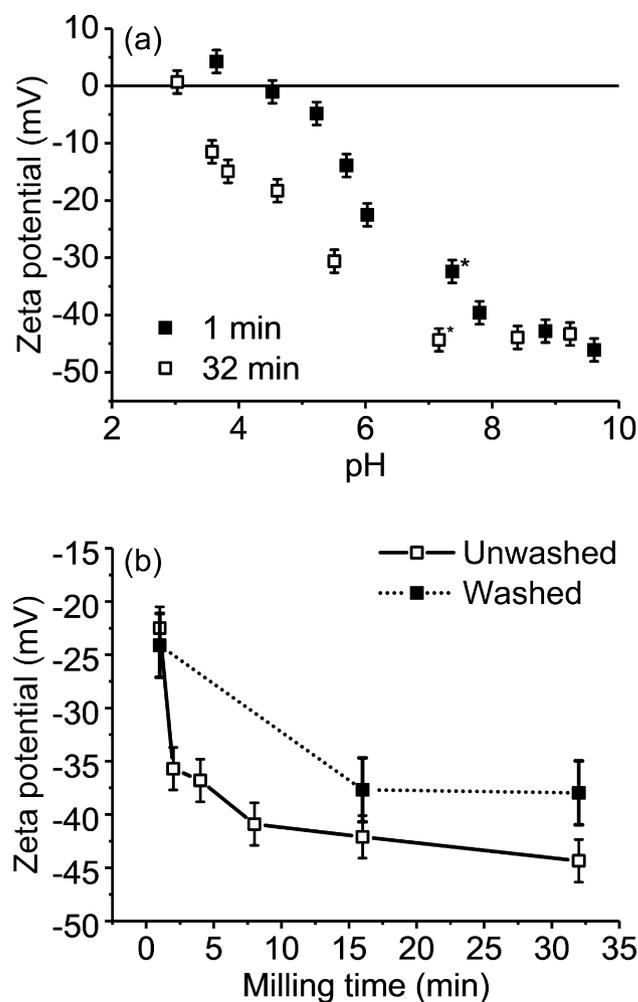
**Fig. 5.** (a) Zeta potential of aluminium doped TiO<sub>2</sub> particles in the presence of sodium hexametaphosphate (SHMP) for 1 and 32 min of milling. The neutral pH is indicated by (\*). (b) Change in the TiO<sub>2</sub> zeta potential with milling time at neutral pH before and after centrifugal washing. In both (a) and (b), error bars represent the maximum standard deviation.
