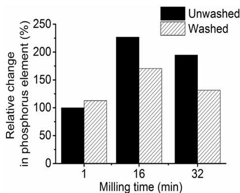
**Fig. 6.** X-Ray fluorescence data showing the relative difference in phosphorus content for 1, 16 and 32 min milled  $\text{TiO}_2$  particles, before and after centrifugal washing. All XRF elemental data was first normalised by setting Ti mass% to 100%. The relative change in phosphorus content with milling time was calculated by setting the 1 min milled sample to 100% phosphorus content.
