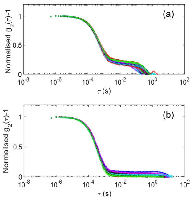
**Fig. 7.** Intensity auto-correlation data from DLS measurements of  $\text{TiO}_2$  suspensions prepared from 1 (a) and 32 (b) minute milled samples. Thirty 30 s measurements were performed for each sample, and each is represented by a different colour symbol.
