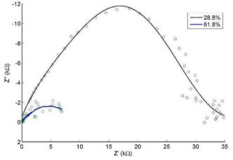
Figure 4, Impedance of digital composite samples of 28.8 wt% and 61.8 wt% carbon loading.
