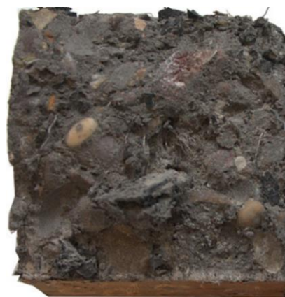
379 Fig. 5 Section through a SFRRuC specimen after 300 days of wet-dry chloride exposure
