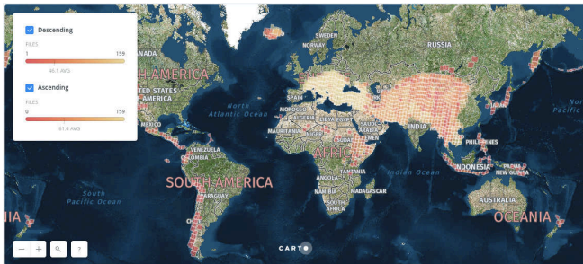
Fig. 2. COMET LICS portal showing number of interferograms processed per frame ( http://comet.nerc.ac.uk/COMET-LICS-portal ).
