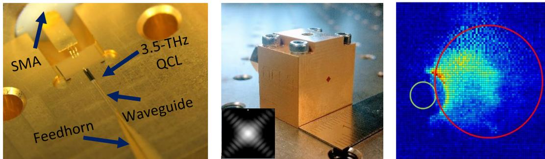
**Fig. 2:** (Left) 3.5-THz QCL mounted within a 150- $\mu\text{m}$ -wide waveguide channel. (Centre) Complete assembled QCL/waveguide enclosure, with diagonal feedhorn aperture visible. Inset: Simulated far-field beam pattern. (Right) Measured near-field profile from Cassegrain optics showing location of primary and secondary mirrors (large and small circles, respectively).
