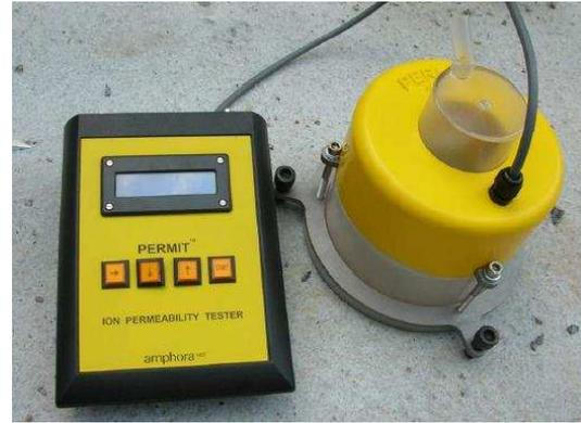
(b) The PERMIT ion migration test apparatus
