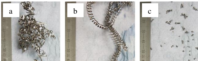
Fig. 3. Titanium cuttings. (a) dry cutting; (b) flood; (c) 60 bar through tool.
