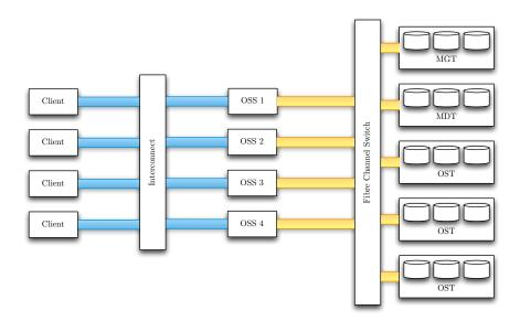
Figure 3.8: An example of a GPFS setup with four OSSs connected via a high performance switch to three targets and separate management and metadata targets.
