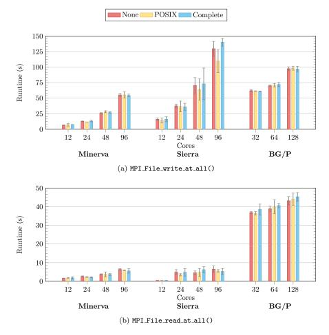
Figure A.2: Total runtime of RIOT overhead analysis software for the functions MPI\_File\_write\_at\_all() and MPI\_File\_read\_at\_all(), on three platforms, with three different configurations: No RIOT tracing, POSIX RIOT tracing and complete RIOT tracing.
