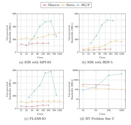
Figure 4.3: User-perceived bandwidth for applications on the three test systems.
