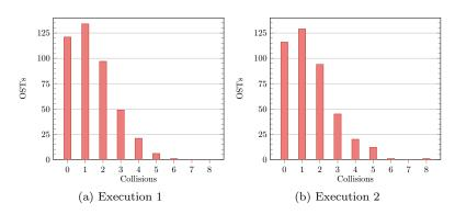
Figure 6.7: The number of OST collisions for IOR running through PLFS with 512 cores.
