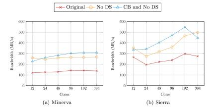
Figure 4.11: Perceived bandwidth for the FLASH-IO benchmark in its original configuration (Original), with data-sieving disabled (No DS), and with collective buffering enabled *and* data-sieving disabled (CB and No DS) on Minerva and Sierra, as measured by RIOT.
