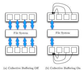
Figure 2.3: An example of two nodes (four ranks per node) writing to a file system with collective buffering off and on.
