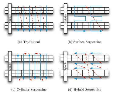
Figure 3.3: Four examples of serpentine sector mapping.
