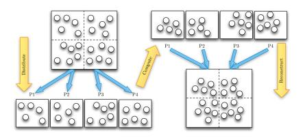
Figure 2.1: An example of the parallelisation of a simple particle simulation between four processors.
