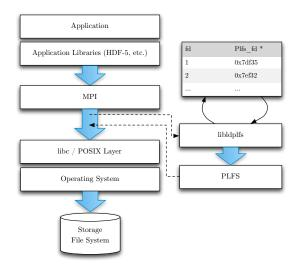
Figure 5.2: The control flow of LDPLFS in an applications execution.
