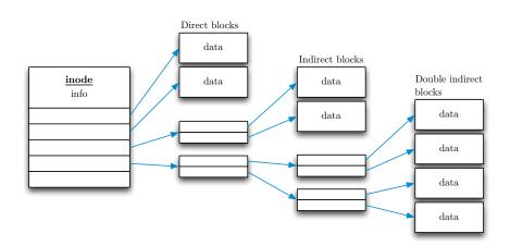
Figure 3.6: Structure of an ext2 inode block.
