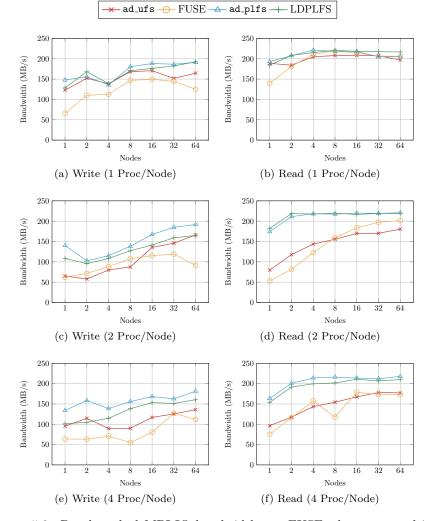
Figure 5.3: Benchmarked MPI-IO bandwidths on FUSE, the ad\_plfs driver, LDPLFS and the standard ad\_ufs driver (without PLFS).
