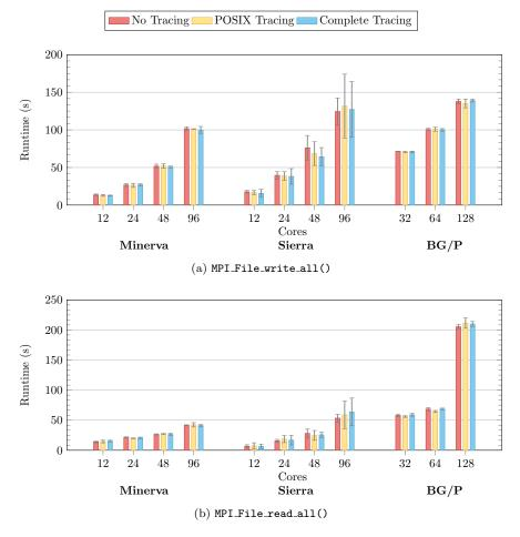
Figure 4.2: Total runtime of RIOT overhead analysis benchmark for the functions MPI\_File\_write\_all() and MPI\_File\_read\_all(), on three platforms at varying core counts, with three different configurations: No RIOT tracing, POSIX RIOT tracing and complete RIOT tracing.
