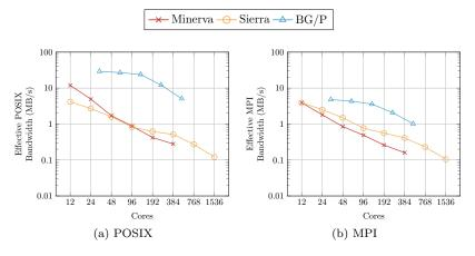
Figure 4.5: Effective POSIX and MPI bandwidth for IOR through HDF-5.
