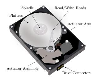
Figure 3.1: Basic internal structure of a hard disk drive<sup>a</sup>. <sup>a</sup>Image includes resources from: http://openclipart.org/detail/28678
