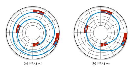
Figure 3.4: An example of four requests fulfilled in-order without NCQ and out of order with NCQ.
