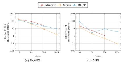
Figure 4.7: Effective POSIX and MPI bandwidth for BT Problem C, as measured by RIOT.
