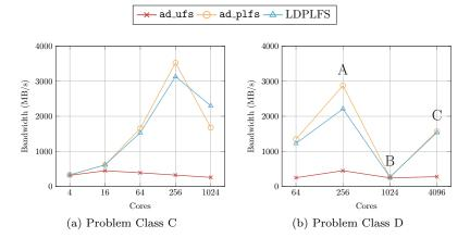
Figure 5.4: BT benchmarked MPI-IO bandwidths using MPI-IO, as well as PLFS through ROMIO and LDPLFS.
