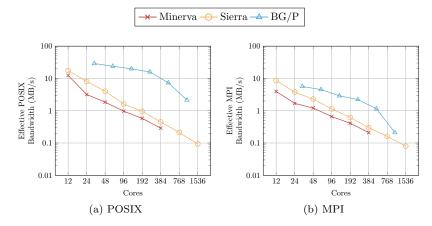
Figure 4.6: Effective POSIX and MPI bandwidth for FLASH-IO.
