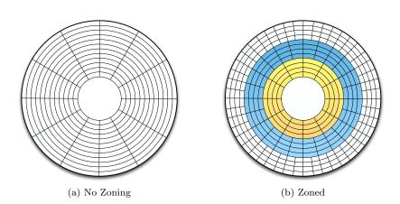
Figure 3.2: Data layout on a disk with no zoning and three zones of increasing density.
