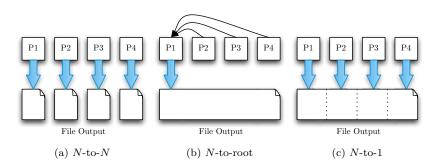
Figure 2.2: The three basic approaches to I/O in parallel applications.
