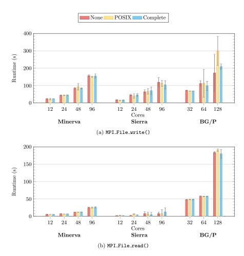
Figure A.1: Total runtime of RIOT overhead analysis software for the functions MPI\_File\_write() and MPI\_File\_read(), on three platforms, with three different configurations: No RIOT tracing, POSIX RIOT tracing and complete RIOT tracing.
