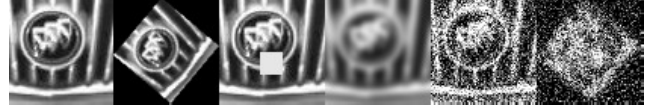
Fig. 7: From left to right are: a testing image, the rotation effect, the occlusion effect, the blurring effect, the noise effect and the combined effect, respectively.
