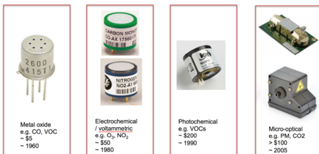
Figure 1. A range of typical low-cost sensor components, example measurement compounds, and approximate cost
