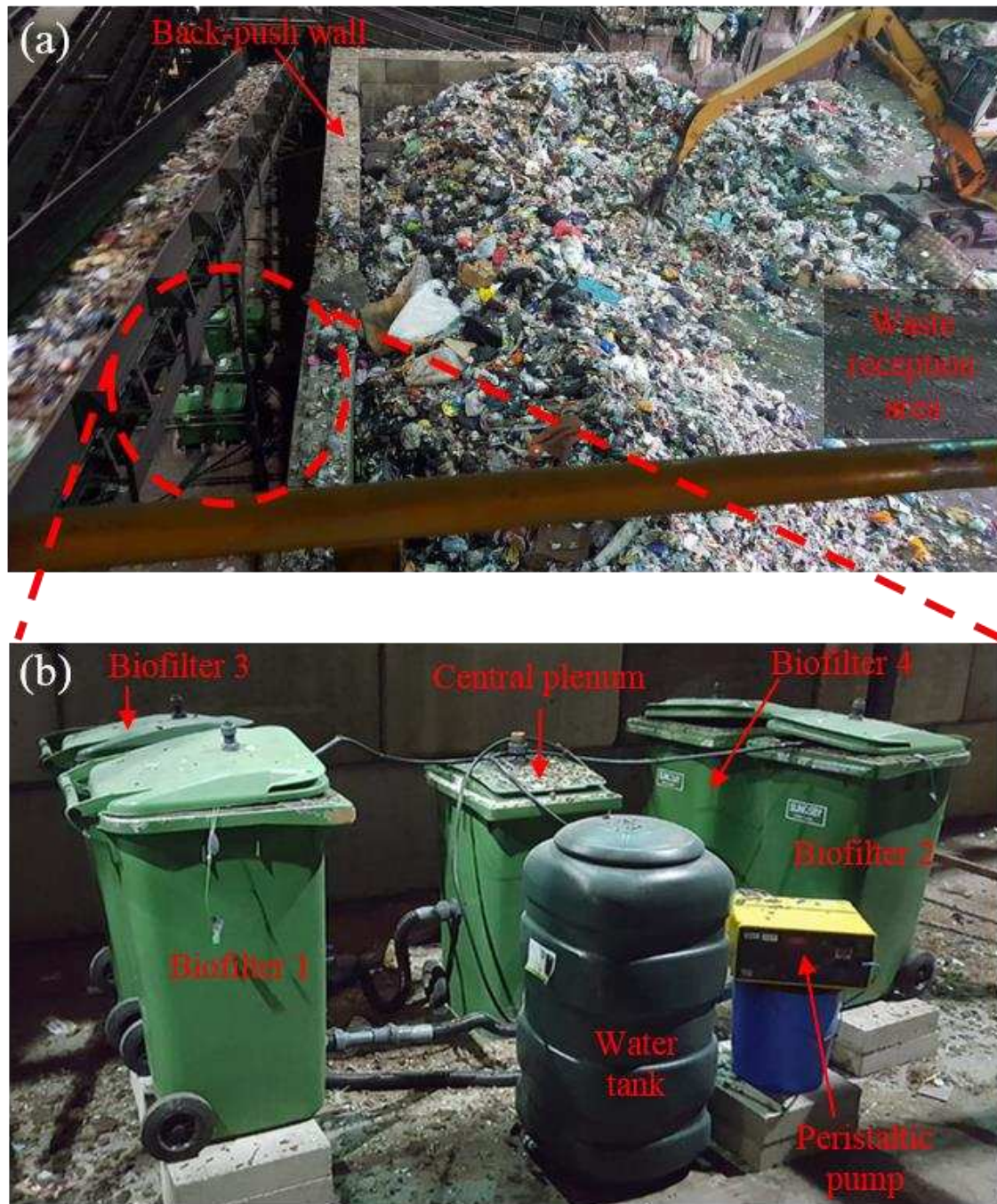
Figure 2: (a) Location of the pilot-scale biofiltration system in the waste hall, and (b) the arrangement of the reactors behind the back-push wall.
