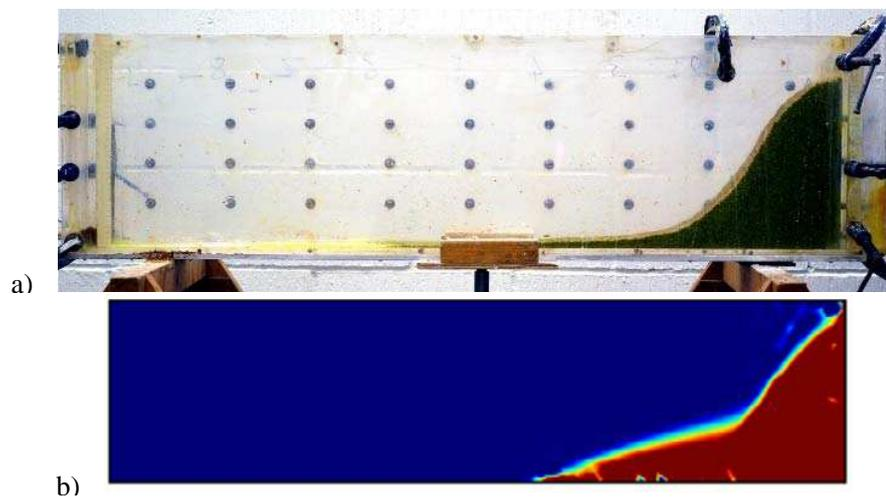
*Figure 4. Grouted sand after colloidal silica injection. a) experimental grouted sand volume, b) finite element model prediction.*
