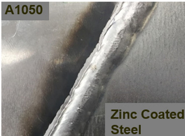
Fig. 3 Spatter-free welding achieved by using EWM coldArc welding technology
