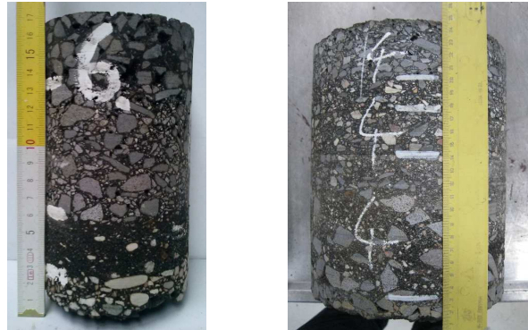
Figure 1. Examples of specimens with layers for which it is impossible to determine the values of their complex moduli in the laboratory
