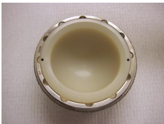
48 Figure 1 Image of a 36mm Pinnacle UHMWPE liner in a titanium shell (left) and a schematic of a cross-sectional unworn 49 rim profile with the nomenclature used in this study (right)
