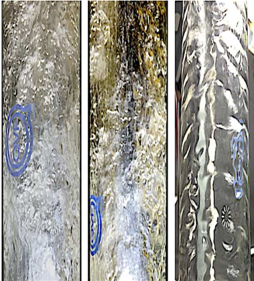
Figure 5: Photography of vertical annular flow, variant 10 (left), 15 (middle) and 20 (right), water film instability as a function of gas superficial velocity
