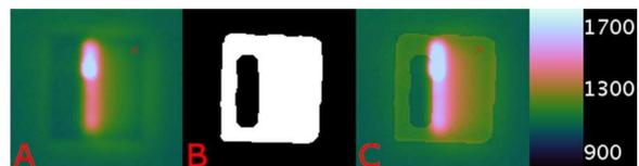
Fig. 10. Images showing emissivity correction by melt pool tracking, temperature scale in K (A) no emissivity correction; (B) emissivity mask; (C) emissivity corrected image Apparent temperature at centre of marked X 1183 K (uncorrected image), 1275 K (corrected image).
