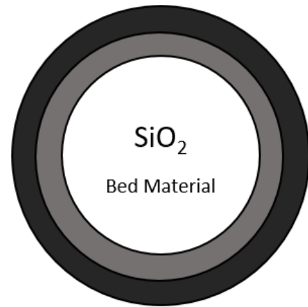
Two-layer coating: K-lean system
