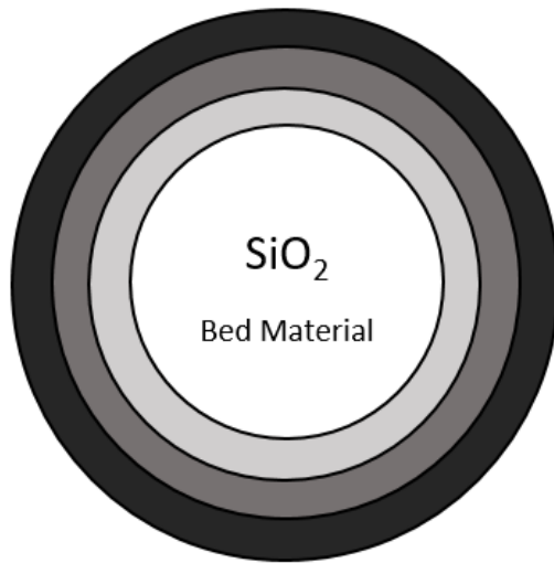
Three-layer coating: K-rich system
