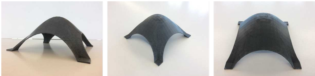
Figure 5 - Additively manufactured plastic shell
