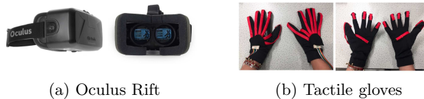
Fig. 3. a) Oculus Rift and b) tactile gloves coupled to the iCub’s eyes and hands, for visual and tactile feedback, respectively.
