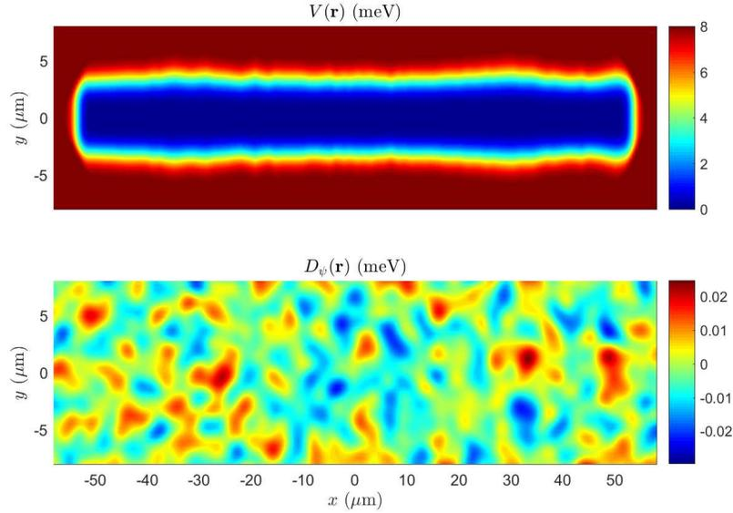
Figure S1. (a) Confining potential  $V(\mathbf{r})$ . (b) Photon disorder calculated with 1  $\mu\text{m}$  Gaussian correlation length.
