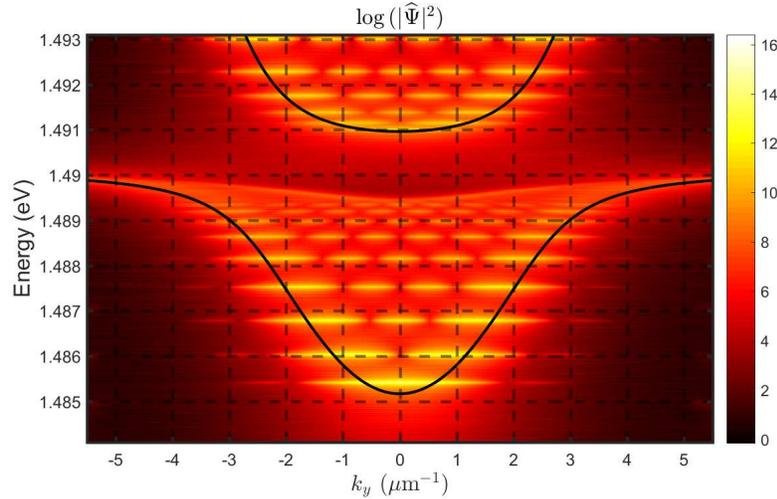
Figure S2. Time resolved dispersion along the  $y$ -coordinate at  $k_x = 0$ . Black solid lines are the analytical upper and lower polariton dispersion curves. Black dashed lines are guide for the eye. Colour scale is logarithmic.
