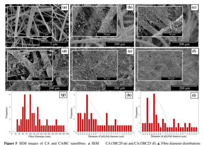
Figure 5 SEM images of CA and CA/BC nanofibres. a SEM image of electrospun CA nanofibre at 15 wt% CA solution. SEM images of CA15BC5 (b), CA15BC10 (c), CA15BC15 (d),
