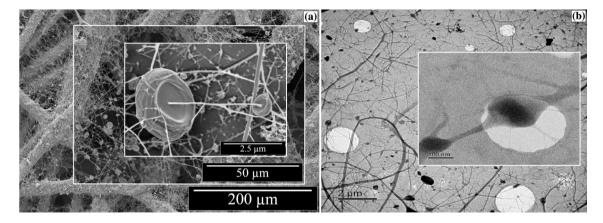
Figure 4 SEM (a) and TEM (b) images of CA nanofibres fabricated from a 15 wt% CA solution with 10 wt% BC/CA loading.
