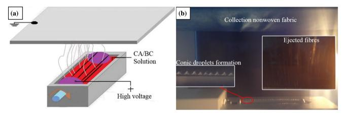
Figure 2 a Schematic of the free surface electrospinning set-up based on a four-wire spindle electrode,  $\mathbf{b}$  real image of the free surface electrospinning set-up using a four-wire spindle electrode
