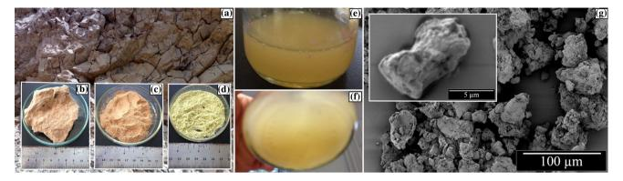
Figure 1 a Naturally occurring BC, b crushed BC, c ground BC, d sieved, purified and activated BC, e, f uniform solution of CA loaded with purified, activated and dispersed BC and g SEM images of raw untreated BC microstones.
