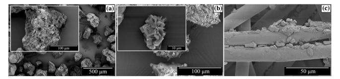
Figure 3 SEM images of a HCl-purified BC, b  $Na_2CO_3$ -activated, HCl-purified BC and reacted with CMC and (AcOH/water) and c electrospun purified and activated BC from (AcOH/water) solution.
