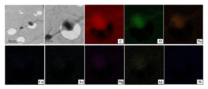
Figure 8 TEM images of 15 wt% CA solution with 10 wt% BC/CA loading and mapping images showing the existence of BC layers, composed of C, O, Na, Ca, Fe, Mg, AL and Si within the CA/BC composite nanofibres.
