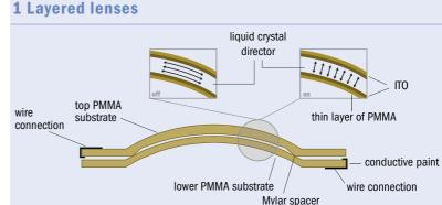
The liquid-crystal contact lenses rely on balancing three layers that act as lenses in their own right.
