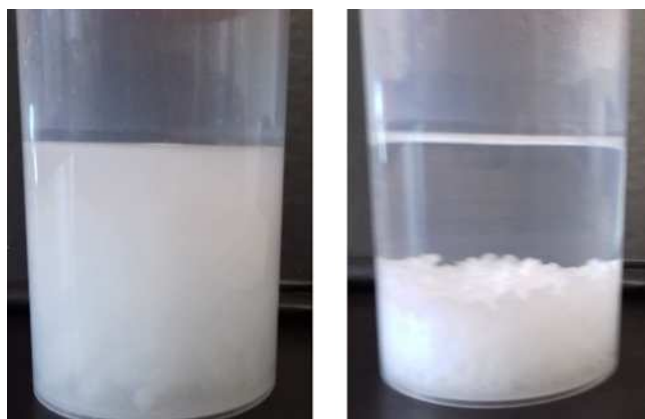
Figure 2: Photographs of silica coagulum in the reaction vessel (a) during and (b) after agitation, demonstrating the solution turbidity and settling that are indicative of an optimal reaction.
