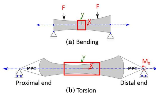
**Fig. 2** Schematic of the bending and torsion loading conditions; **a** Four-point bending: two equal forces applied to the femoral shaft, adapted from Li et al. (2015); and **b** Torsion: moment around the  $x$  axis was applied at the distal end while the rotational movement of the proximal end was fixed in this direction. Regions of interest for both bending and torsion are highlighted in the red boxes
