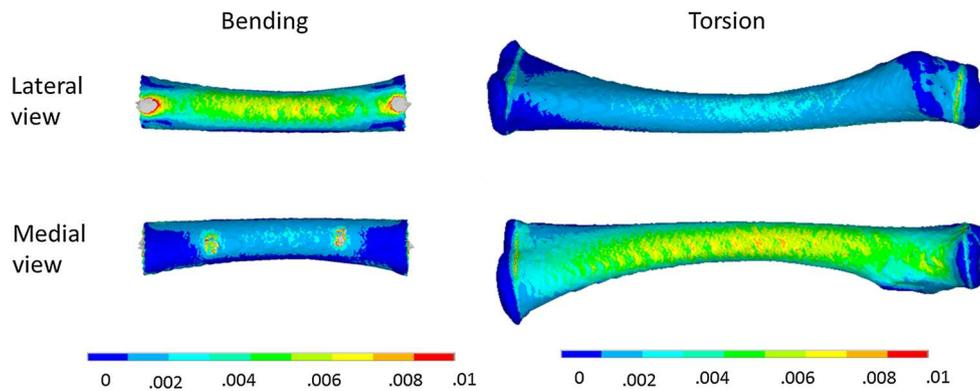
**Fig. 3** First principal strain distributions under bending and torsional loads are shown in the lateral and medial views. The illustrated femur model was obtained from a 1-year-old. The direction of loading was
