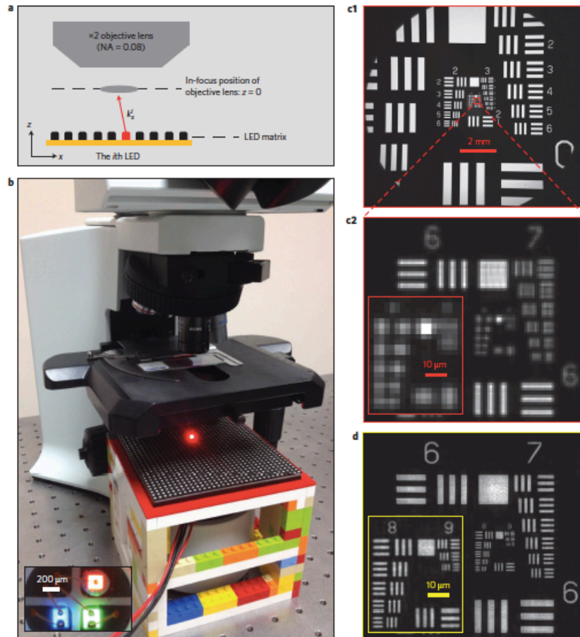
Figure 28: A Fourier ptychography microscope, shown schematically in (a). (b) A conventional microscope has been modified using a Lego framework so that an array of photodiodes can illuminate the object at different angles (see bottom Figure 26). (c) A
