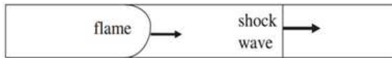
Fig. 1: Flame and shockwave propagation in an open ended tube. Ignition initiated from the closed end [1].
