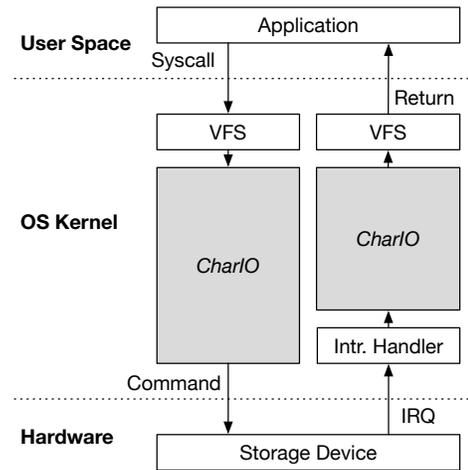
Fig. 2. Storage access layers using CharIO driver
