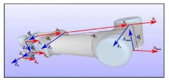
Figure 1. The Definition for centre of mass parameters [1]
