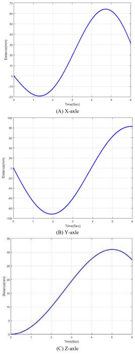
Figure 2. Trajectory of tool mounting bracket (Joint 7)
