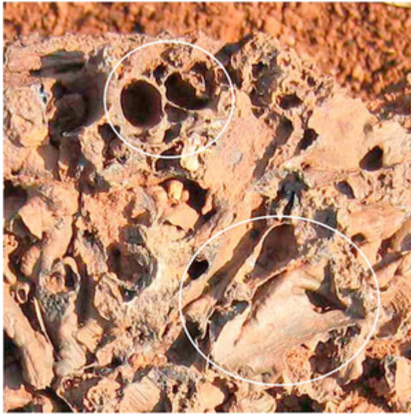
Figure 7. Slag fragment from western Uganda. White circles indicate the position of reed impressions preserved on the slag surface.
