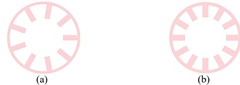
Fig. 14. Stator geometries. (a) 9-slot. (b) 12-slot.
