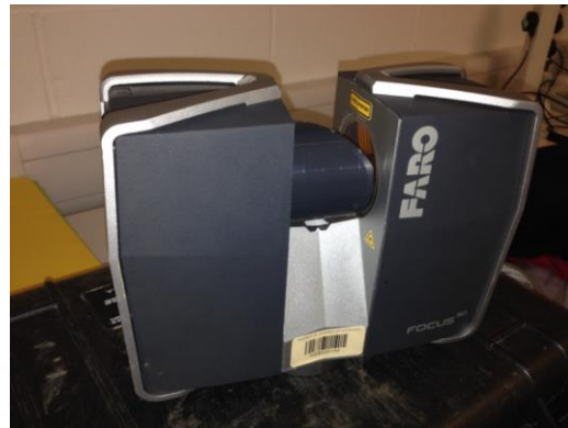
Fig 4. The front view of the laser scanner FARO Focus 3D
