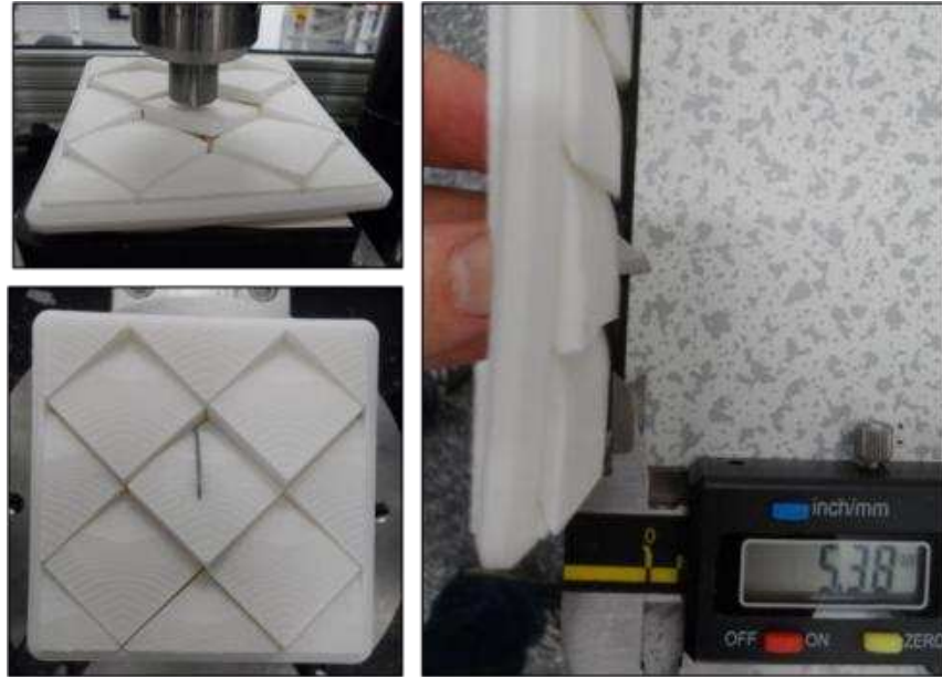
Figure 8: Measuring blade penetration on Imbricated Assembly Two.
