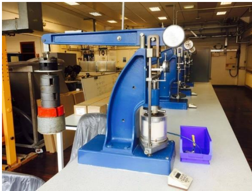
Figure 6. The test equipment showing the loading frame and consolidation cell
