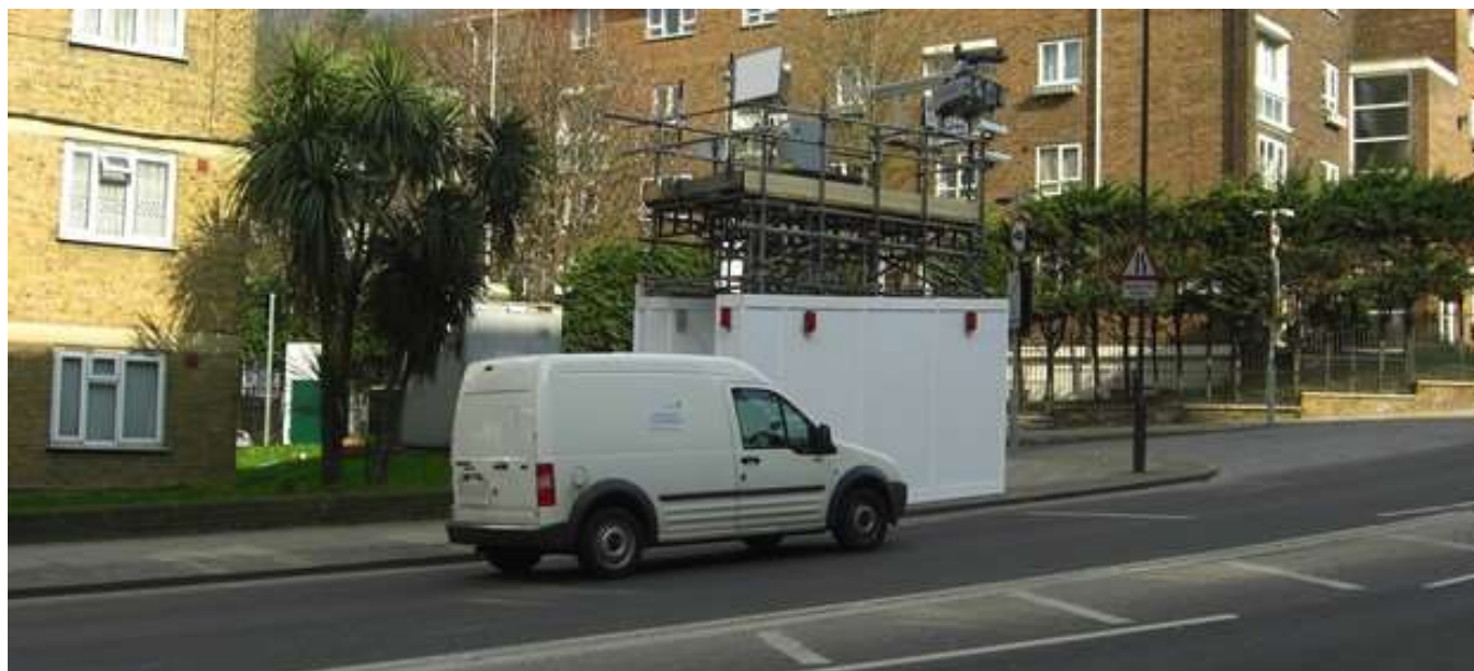
Figure S2: EDAR deployment at Greenwich Blackheath Hill as part of the UoB/UoL/KCL study. Left, the EDAR deployed on purpose-built scaffolding at the roadside, with the EDAR installed at 5 meters nearby rather than directly over the road and traffic flows. The same photograph also shows the PEMS vehicle approaching the reflector strips where EDAR exhaust emission measurements are made and (behind the scaffolding) the local air quality monitoring station. Right Top and Bottom, the two EDAR units (one for gaseous species, one for PM) and the speed and automatic number plate capture cameras, respectively.
