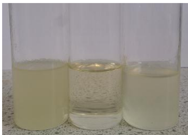
Fig. 8. The reverse emulsions were synthesized with adding 0.5 g of different (at pH=7 and 40 wt% of Span80), a,b) polymer cosurfactant mixing, c,d) alcohol and diol cosurfactant.
