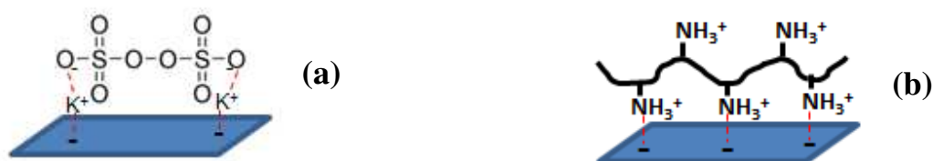
Scheme 2. Schematic illustration of (a) KPS-MMT ionic interaction, and (b) chitosan-MMT electrostatic interaction.
