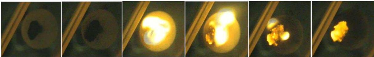
**Figure 3. Frames from the devolatilization and ignition step of El Cerrejón coal.**
