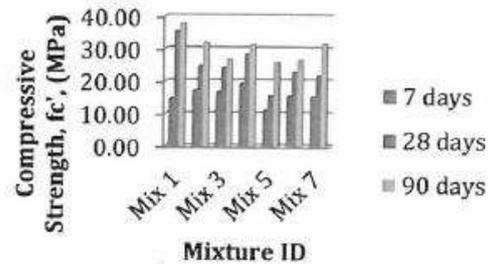
Figure 1: Compressive strength of the concrete samples
