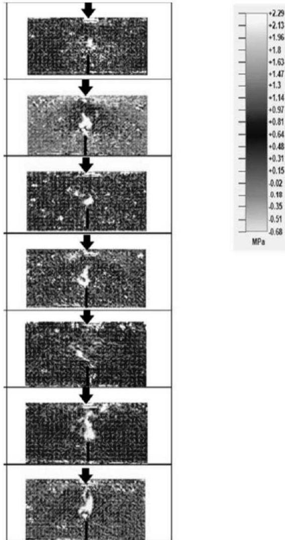
Figure 3: Flame-like distribution of maximum shear stress ahead of the notches on the notched samples 1-7 under the ultimate load (top most sample ID is 1 and bottom most 7 in the ascending order. The notch at the middle is shown in black colour in the plots. The short arrows show the direction of the major principal stress)
